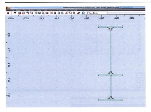
Section geometry should be placed in the coordinate system center. It can be done by selecting contour and using Edition > Translate option
