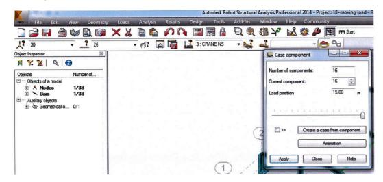
Vehicle position can be seen after switching on Moving loads option in View > Display> Loads dialog box
