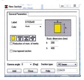
Once the **New Section** dialog box is closed, the recently defined section is available in the **Section** field of the **Bars** dialog box. Set the cursor in the **Node Coordinates** field and enter the following points coordinate in the **Beginning** and **End** field:
