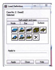
Click the *Uniform Planar Load* icon and introduce the load value pz = - 5 (kPa) into the new dialog box (see the picture below),
