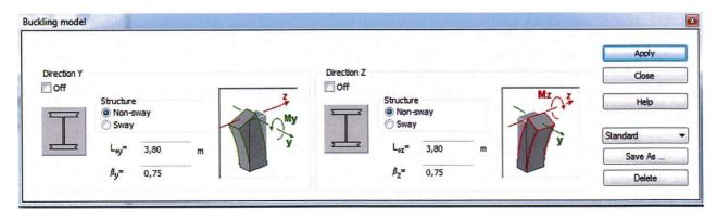
Each of those parameter sets can be saved and assigned to dimensioned column. The best way for parameters assigning is use of **Object inspector**
