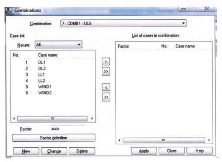
Press the **Factor Definition** button and set the arrow to point the *CAT A* label. In the *Factor* edit field introduce the new value 1.55 and confirm by clicking **Change** button. Close the dialog box by pressing the **Close** button.
