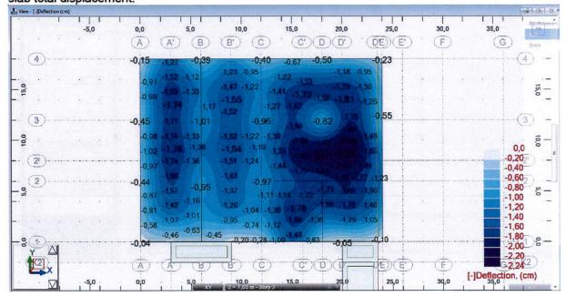
More accurate results can be obtained with use of deflection **Verification with stiffness update.** Verification with stiffness update can be done after selection of critical (for deflection) SLS combination case. Usually one can choose combination with maximal static displacement for designed element.
