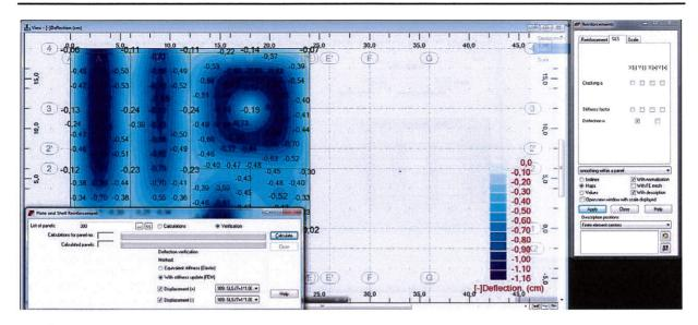
Reinforcement maps and reinforcement tables can be saved with use of Screen Capture option and then edited in Printout composition module.
