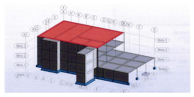
While dimensioning parameters definition one has to determine main reinforcement direction. In that case local panel coordinate system can be used. If main reinforcement direction will be set to **Automatic** it will be parallel to local panel X axis. In results AX area will be presented for reinforcement parallel to panel local x axis AY for reinforcement parallel to panel local Y axis.
