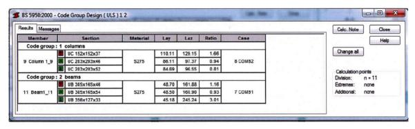
Launch calculations. The program will carry out the design calculations with section optimization. From a set of sections, the program selects the most optimal one with respect to weight. Clicking the *Change All* option results in exchanging the section applied during the design process for the optimized sections.
