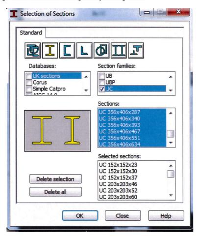
In order to create the second group, one should click the **New** button, and type *Beams* in the *Name* field. In the *Member List* field enter the beams numbers (i.e. 10,11). By clicking the **Sections** button, make the sections: *UB* available for verification. Close the dialog box by clicking **OK**. Save the settings by clicking **Save**.
