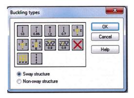
By clicking the appropriate icon, one should select the coefficient 1.0 (first icon from the left in the first row). Once the selection is done, close the dialog box by clicking **OK** button. Then, perform the same operation for direction **Z**.
