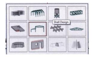
Change structure type to shell by selecting the *Shell Design* option (the third one from the left in the second row).
