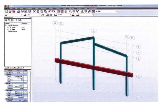
While information about elements are transferred program asks about loads transfer way (simple cases or manual combinations). Simple cases mode uses default code combination regulation for combination definition so user defined coefficients are not taken into account. In our model one should use manual combination option.
