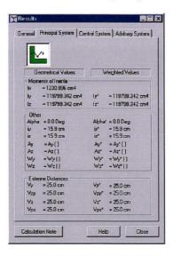
Click the Calculation Note button in the bottom part of the Results dialog box (or select the Results / Geometric Properties / Calculation Note command from the main menu) to generate a calculation note. To save the section in the user's database: one should select the File / Save to Databases command
