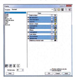
The available tabs allow one to get access to the data on structure parameters. This option is also available from the main menu by means of selecting the *View / Display* command.
