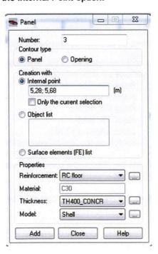
To define new thickness, click the \_\_\_\_ button to the right of the *Thickness* field and set the appropriate values in the dialog box that appears after clicking (see the picture below).
