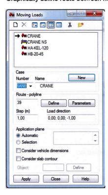
In the same way moving load case for non symetrical crane can be defined
