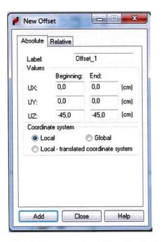
In the Label field enter the name Offset\_1 for new offset. Then in the UZ field introduce the offset value (in the exercise the offset value is equal 45 cm as it is half of RC slab height plus half of RC beams
