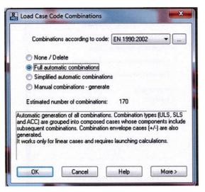
This option allows for definition and modification of code combinations. To define load cases for combination:
