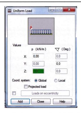
apply defined uniform load to structure spans (bars 4,5,6,7,). Go to the Apply To field in the Load Definition dialog box; the mouse cursor will change from the choice mode into the selection mode. Then, indicate beams 4,5,6,7 in the graphical viewer (with the Ctrl button pressed, click on the bars). The bar numbers will appear in the Apply To field. Confirm the selection by pressing the Apply button
