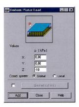
Confirm the settings pressing the **Add** button. In the *Apply To* field enter the number defining the plate to which the load will be applied. Finish the operation pressing the **Apply** button and then close the **Load Definition** dialog box pressing the **Close** button.
