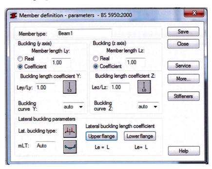
In the *Buckling length coefficient* field select the coefficient for directions **Y** and **Z**. To achieve this, one should click the icon, which results in the appearance of the dialog box (see the picture below) that allows one to select the buckling length coefficient.
