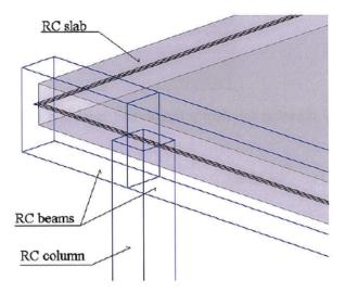
In order to define offsets select from the menu *Geometry / Additional Attributes / Offsets*, this opens the Offsets dialog box. From the upper toolbar select the icon (*New*). A dialog box for defining new offset will be open.
