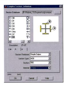
Confirm by pressing **OK**. A section consisting of two I-sections will appear in the graphical viewer. In order to generate the results, choose both contours (**CTRL+A**) and then select *Results / Geometric*
