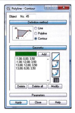
One may also defined the contour by introducing appropriate coordinates manually in the Geometry field.
