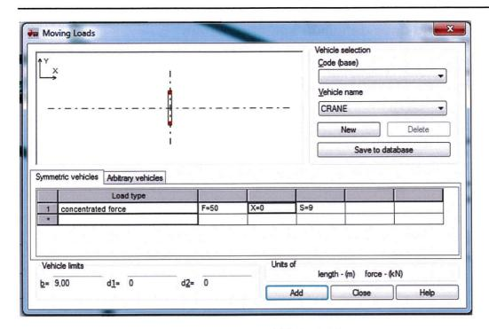
Then Add option should be used to save new vehicle in database
