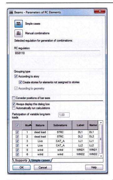
While beam and column with selected loads are transferred to provided reinforcement module they can be selected for dimensioning in Object Inspector
