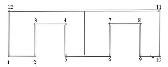
Select from the menu *Geometry / Objects / Polyline-contour* command that opens the *Polyline-Contour* dialog box. In the *Definition Method* edit field select the *Contour* option. Place the cursor in the *Geometry* field and introduce coordinates of the points defining the appropriate contour:
