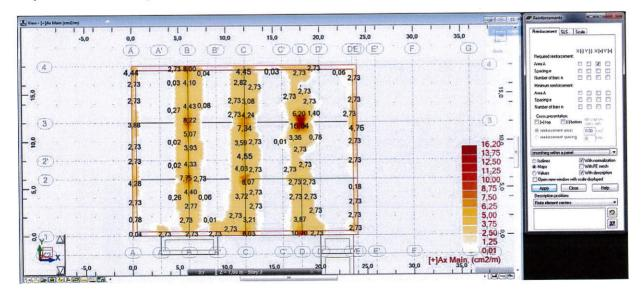
Results can be presented in reinforcement table (Design / Required reinforcement for Slab/Walls Option / Table Plate and shell reinforcement).
