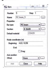
Select *RC Beam* option in the *Bar Type* field of the *Bars* dialog box. Click the \_\_\_\_\_ button located to the right of the *Section* field. This results in the appearance of the *New Section* dialog box (shown on the picture below) and define a concrete beam with the section dimensions 200x400. One should set the following parameters in the dialog box:
