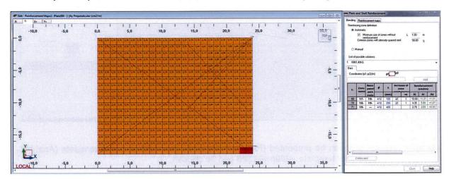
Bottom reinforcement in Y direction
