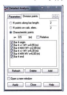
Select case 7:COMB1 in the Case Selection combo-box. Go to the Detailed Analysis combo-box and press the **Refresh** button and then the **Apply** button.
