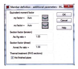
Define the Ae/Ag r Ratio = 1,0 in the Sections Parameters field
