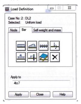
Define uniform loads pz=-25 kN/m for roof beams 11, 12
