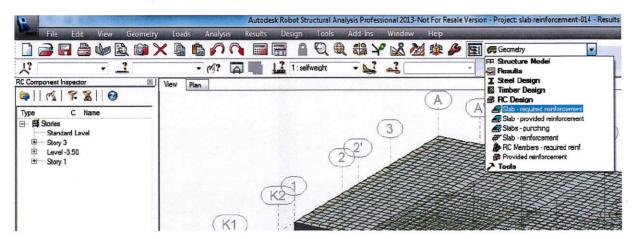
After story 3 lab and staircase wall selection one can use "<<" in Plate and shell reinforcement window to calculate reinforcement for selected object only. Then Calculate can be launched. For objects calculated with compression/tension option on, Method- analytical should be used. Option Reduction of forces at supports and above columns and walls should be checked on to avoid reinforcement concentration above supports
