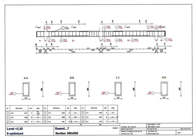
While beam drawing is edited one can choose generate sections position and change drawing scale.
