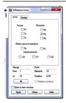
After choosing element number position and internal forces type we can Apply and obtain diagram
