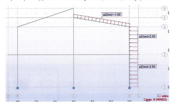
Loads can be modified graphically or in load table. Go to the *Loads* table. The *Edit* tab allows one to modify the existing loads and define new ones.
