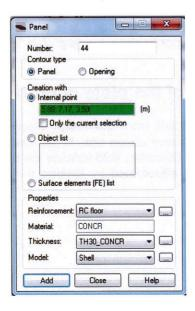
Set the reinforcement type for *RC\_floor* in the *Reinforcement* combo box. Select the thickness *TH300\_CONCR* from the *Thickness* combo box in the *Panel* dialog box and then, set the cursor in the *Internal Point* field. Move the cursor to the graphical viewer and indicate once a point within the boundaries of the rectangular plate.
