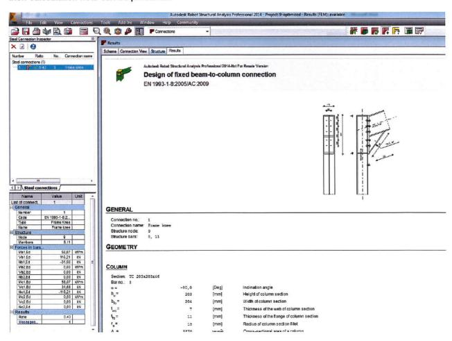
Another connection can be defined by switching to Structure tab selecting connection node and adjoining elements and clicking "New connection for selected bars" option
