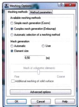
Select from the menu the Analysis /Meshing/Local Mesh generation command. If this option is selected, *Autodesk Robot Structural Analysis* generates the calculation model of a structure (finite elements).
