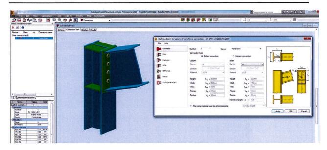
Steel connection module does not optimize connection. User can modify connection parameters defining bolts distibution, additional brackets and stiffeners then verify connection
