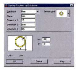
Confirm the operation clicking the **OK** button, the section is saved to the database.
