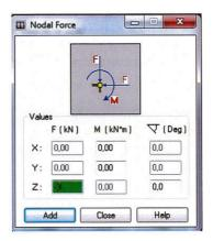
It is also possible to define loads in the relevant table. To do so, one should go to the layout of loads by indicating *Loads* option in combo-box in the top right corner. Once the layout changes, one should define appropriate load types and define their values in the table.
